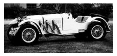
The engineering of the SJK is outstanding, as befit a Mercedes-Benz. The 1.49 liter six-cylinder engine turns out 40 brake horsepower, wich is well complemented by precise steering.
