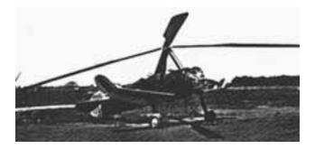
The Pitcairn autogyro is the most popular autogyro available. This air vehicle is a rotary wing aircraft which is noted for its extremely short take-off distance. By gearing the engine to the rotor and then disengaging it once airborne, it can take off and land from the roof of any large building. Almost a helicopter, it lacks only a helicopter's ability to hover. Numerous adventurers and the Shadow have made it the air vehicle of choice. With external tanks, it range can exceed 186 kilometers.
