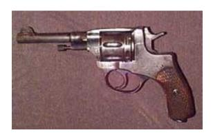
The Nagant gas-seal revolver was patented by the Nagant brothers (Emile and Leon) in 1892 with some additional improvements made in 1895. This design was one of several offered to the Imperial Russian Army as a new service revolver in 1895. Emile and Leon were on good terms with the Russian Army due to a previous cooperative effort to produce the Mosin-Nagant M1891 service rifle. This may be why the Russians adopted their design.
