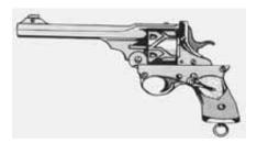
This is a unique revolver possessing a very distinctive design. When fired, the force of the recoil turns the cylinder automatically, making it effectively a semi-automatic revolver. The Webley-Fosbery is also an early user of speed-loaders. (same as the Webley).
